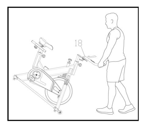
Firmly grasp and hold each side of the **Handlebar (No.18)**. Place one foot on the front base and tilt the bike towards you until the transport wheels on the front base touch the ground. With the wheels on the ground, you can transport the bike to the desired location with ease.
