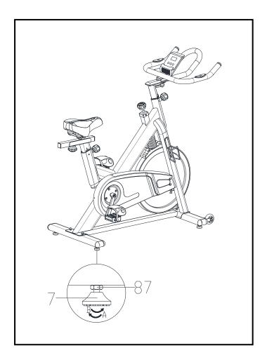
To achieve a smooth and comfortable experience, you must ensure that the bike is stable. During use, if you notice that the bike is unbalanced, you can adjust the **Base Levelers (No.7)** located beneath the **Front and Rear Stabilizers (No.2 and 8)**.
